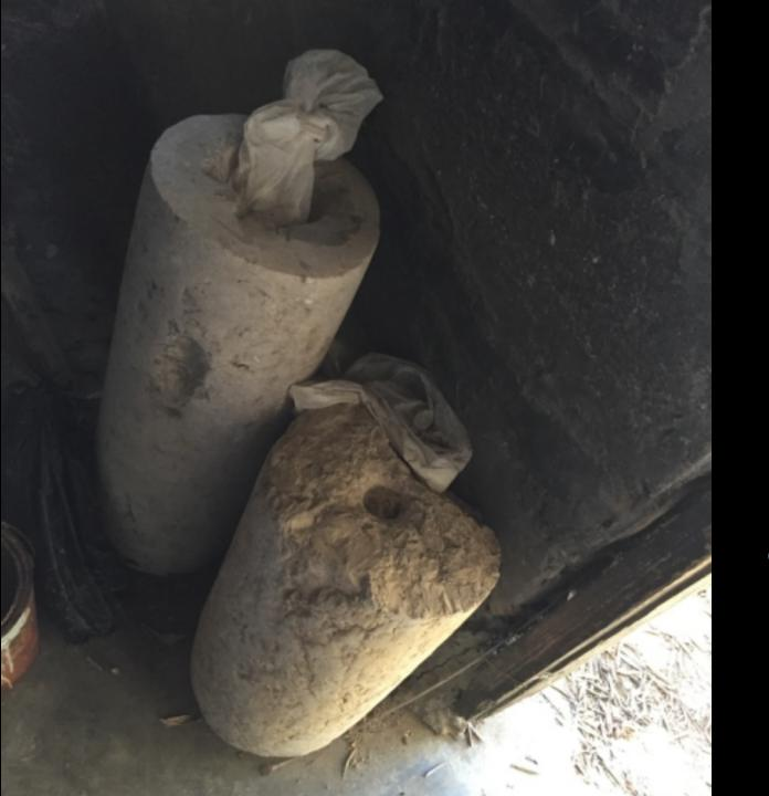
**STONE CYLINDERS WERE USED TO ROLL** DIRT OVER ROOF, TO **PROVIDE FOR** THERMAL ISOLATION
